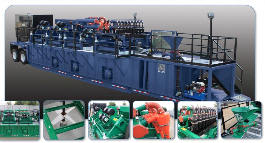
9,000 gallon triplepartitioned tank with continuous recirculation dewatering system.
