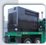
200 KW On-Board Generator Package
