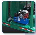
Diesel powered hydraulic jacking system to level the system upon placement.
