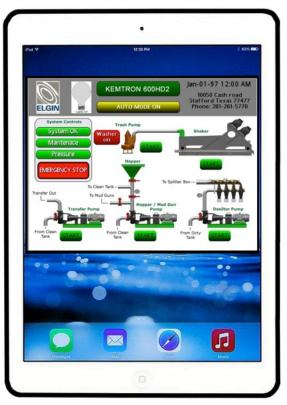
Run Time Counters Will Preemptively Notify Operators of Greasing and Maintenance Schedules. Detailed Event Logs Will Track Fault Conditions and Maintain Detail Records of the Units Operation. On-Board Hydro-Cyclone Pressure Sensors Will Notify Operators of Need to Service Equipment. Any Tripped Electrical Conditions Due to Overloads Will be Clearly Noted on the User Interface. Full Wireless Integration with Your Smart Phone or Tablet with a Dedicated Local Wifi Network.
