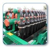
Includes forty (40) 4", ceramic-lined desilters with screen savers & valve isolation.
