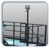
Two sets or retracting deck lights fully illuminate the working deck of the entire system.
