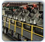
Six (6) Six-Panel Dual-Deck Linear Motion Shakers with **340 ft²** (**31.6m²**) of surface area.
